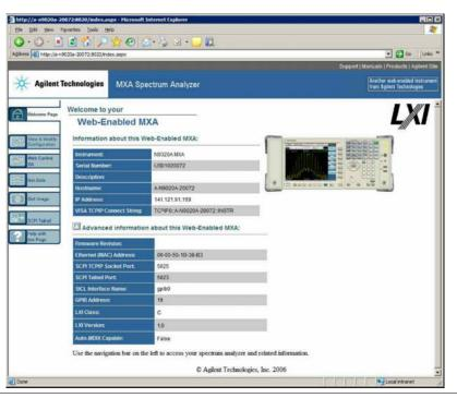
At the left side of the page are a set of tabs that provide access to configuration information for the instrument, plus the ability to control it through the web interface.
