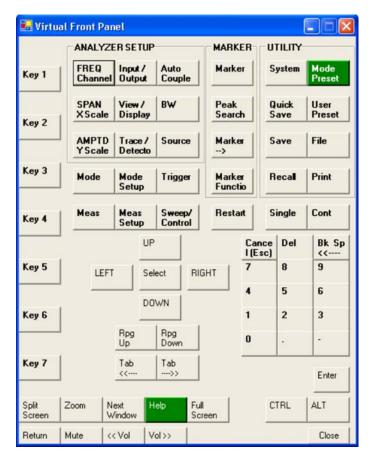
When you click a button in the Virtual Front Panel, it performs the operation of the corresponding instrument front-panel key. The buttons at the left of the panel, named Key 1 through Key 7, perform the operation of the respective softkeys. The Rpg Up and Rpg Down keys perform the operation of the knob.
