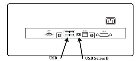
In addition, the Agilent IO Libraries CD that was included with your instrument contains USB Host drivers that allow control of other instruments connected to the USB bus.
